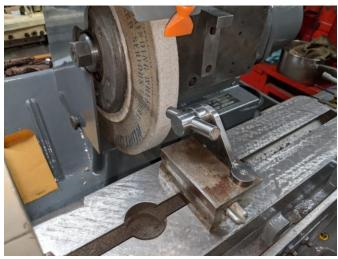
he showed two tools he is going to make for the grinder, a Centring (their spelling) Sleeve and an ID grinding stone adapter. Both will be made from pre-hardened 4140 obtained from McMaster-Carr.
