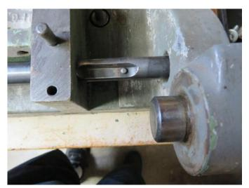
conjunction with the square part shown below which sits in a >90 degree crotch on a large lever arm. This square piece can rock in the crotch as the notched shaft is turned. The notch in the shaft is off center so when it turns it supplies cam like motion pushing down on the little cube as it rocks in the crotch. Opposing forces then keep the shaft in position in the clamped mode.
