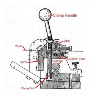
finding a good manual for it but did find very useful drawings for the mechanism in the patent drawing shown above. The following pictures show the base, hinge assembly and bearing plate. Note the nice beefy nature of these castings. This is no surprise considering how solid and smooth these old tools are in operation.
