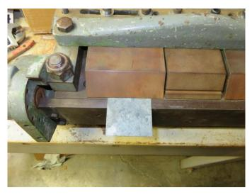
spring on the side of his brake that keeps the adjustable table snug up against the adjustment screws. Not all the members with these tools recalled seeing this spring. He wanted to replace the spring, so he found a good candidate on eBay but had to make a new set of standoff-mounts to accommodate the style of spring that he purchased.
