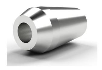
The centering sleeve will have a 2MT socket and a custom 12 Degree outside taper to fit the Myford work head.
