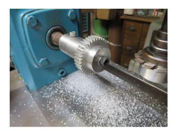
output display and to control a stepper motor to drive the indexer. He used the tool to make a pair of gears and found it to be quite accurate. Dan showed some slides of the tool and a short video of the gear cutting operation. He passed around the gears for inspection.
