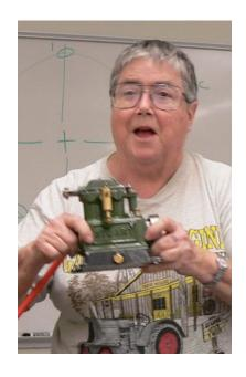
Stuart steam engine with the help of Frank Kerpsie and his compressed air tank. Pat said this engine is not a model, but a small engine built to power a generator for charging radio batteries on remote island outposts during WWII.
