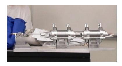
Graham Hollis showed the progress on the Snow Engine he is building. He has completed the base, supports, cylinders and valve works. Graham's workmanship is superb and this engine is beautiful, all polished aluminum and steel. He is working on this very ambitious project as a diversion from his efforts on the sleeve valve radial engine he is also building. Graham likes to keep several irons in the fire.
