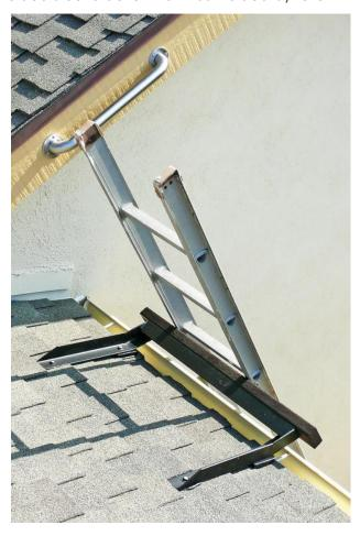
club member Bernie Wasinger. This was actually built some years ago. With the brace in place an extension ladder can be safely and securely laid in place without concern for crushing the rain gutters. Once at the top of the ladder, he added a grab bar to the closest facial board. This was one those chrome plated U-shaped steel handles typically used in bathrooms for older folks. This gave him a firm handle to grip at the top of the ladder as he transitioned to and from the roof.
