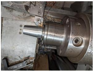
Once the basic shape was in place, he transferred the sleeve to the OD/ID grinder to first clean up and accurately grind the 12 degree outside taper.
