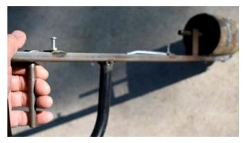
the ladle out of an old propane bottle and welded up a handle and mechanism to hand operate the valve he made for the bottom opening. He melted up a batch of aluminum scrap and poured the molten metal into a cast iron muffin pan to make a bunch of little ingots. He found that any clogging of the valve was quickly resolved by dipping the ladle back into the molten metal. It was an impressive gadget and should prove to be very useful.
