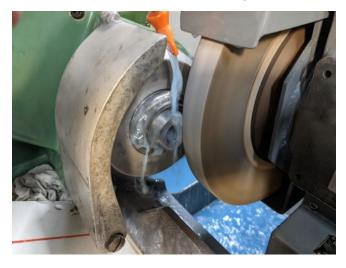
socket to final dimensions and grind the face of the sleeve. The image below shows the final part.
