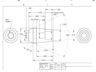
the part he created in Onshape based on images of the sleeve he found online. He then proceeded to turn the rough dimensions from a piece of 1-3/4" pre-hardened 4140 which has a Rockwell hardness of C25. The turning operations were all carried out on the lathe including the internal threading using carbide inset tooling.
