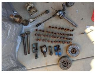
workhead and a batch of accessories he later bought on eBay for it. The Myford workheads (similar to a headstock on a lathe) have a special 12 degree included angle socket. He needed to make an adapter to convert from this 12-degree opening to a standard 2MT socket for inserting dead centers. Myford calls this adapter a Centering Sleeve. He presented a pdf drawing of
