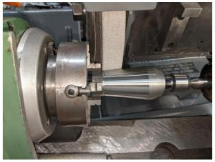
Once this was complete, he removed the four-jaw chuck from the headstock and inserted the new sleeve. At this point he was able to grind the 2MT
